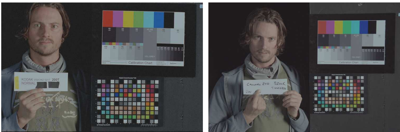
Figure 5. A reference image from the film scanner (left) and a still image transformed using a second order polynomial model (right)
